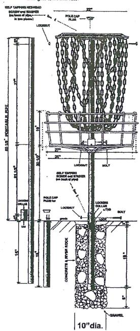
POLE (66 in.) - 1 1/2 in. (.D., 1 15/16 in. O.D. hot-dipped galvanized pipe, drilled
