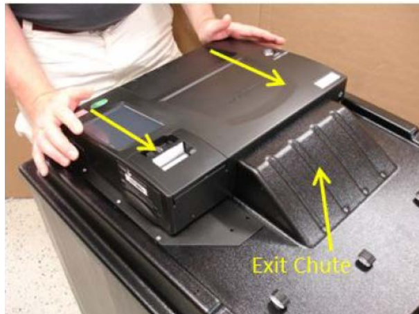
Figure 6-2: Position the tabulator on top of the ballot box
