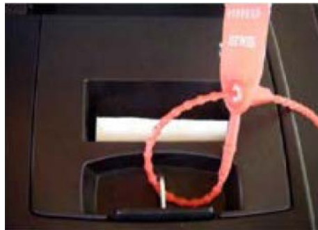
Figure 6-7: Sealing the Thermal Report Printer Door
