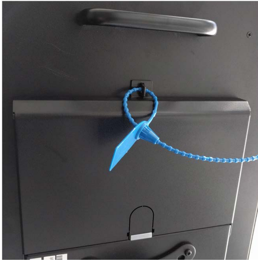
Figure H-16: Top security latch plastic sea
