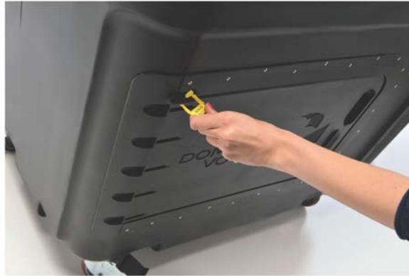
Figure 6-111: Breaking the Ballot Box Seal
