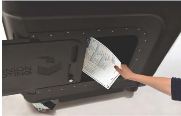
Figure 6-94: Removing Ballots from the Ballot Box
