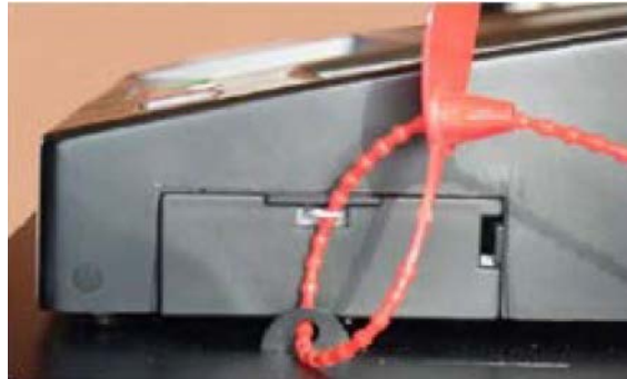
Figure 6-8: Sealing the Modem Port
