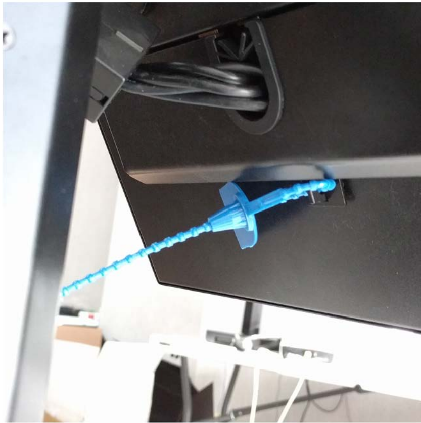
Figure H-17: Bottom security latch plastic seal
