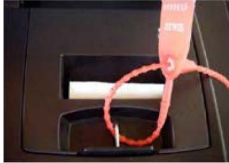
Figure H-11: Sealing the thermal report printer door
