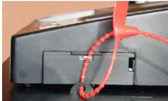
Figure H-12: Sealing the modem port
