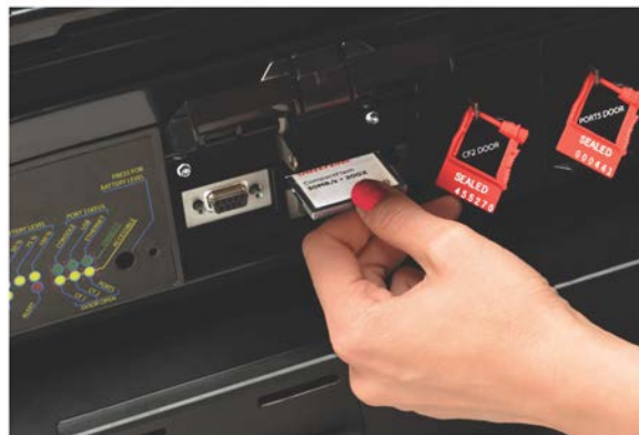
Figure 6-95: Removing the CF1 Card
