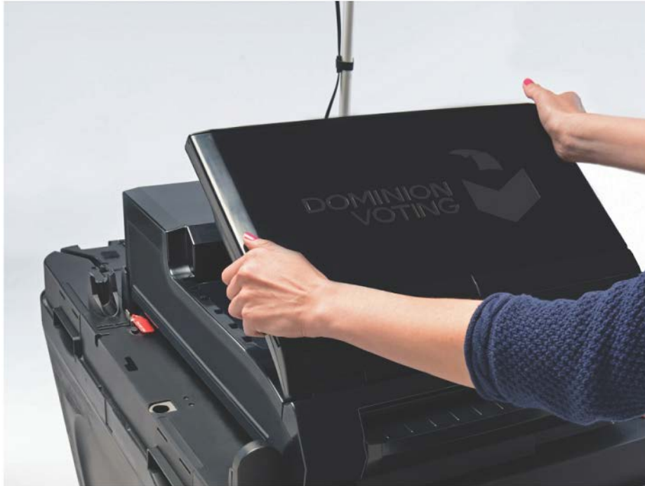
Figure 6-15: Lifting the LCD Screen on the ImageCast ® Evolution
