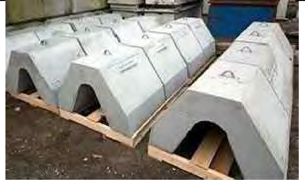
6" PIPE ANCHOR DETAIL 2/12
