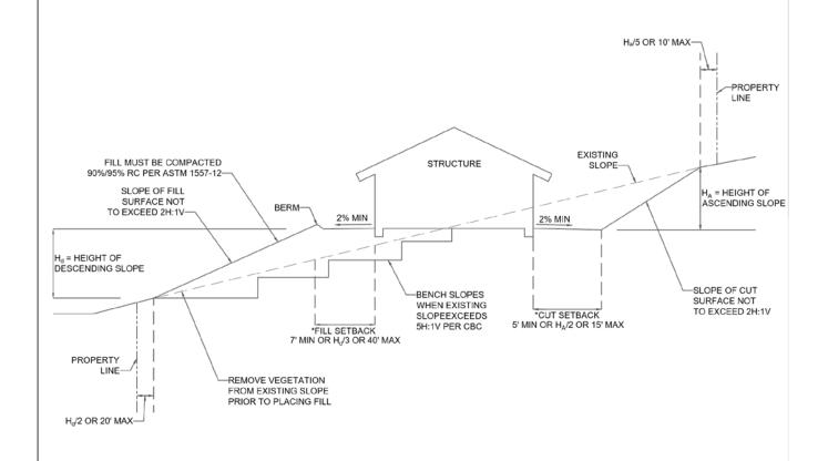
\* SPECIAL SETBACKS DO NOT APPLY WHEN CUT, FILL, OR EXISTING SLOPE FACES ARE 3H:1V OR FLATTER
